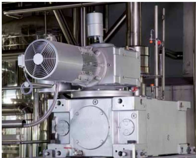
A single motor controls the lautering process: It is used to loosen and slice the spent grain but also to remove it, namely to empty the tun after the process is completed.
