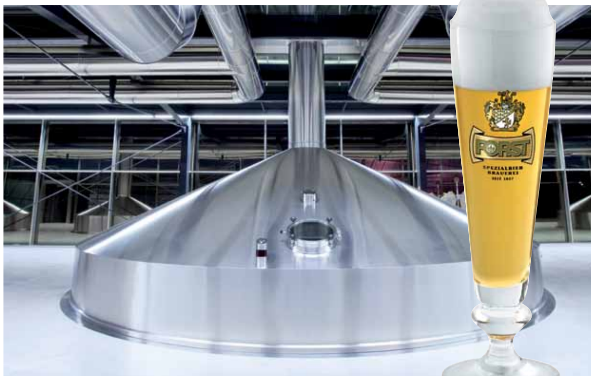
With a diameter of 8.6 metres, the lauter tun forms the heart of the brew house.
